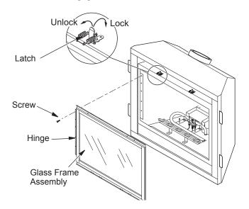
Figure 42 - Removing/Replacing Glass Door
